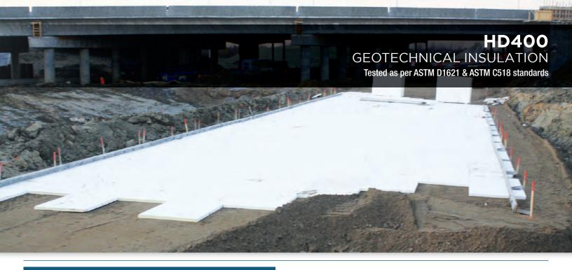
VERY HIGH DENSITY, compression resistance 414 kPa / 60 psi (When tested at 10 % of deformation as per ASTM D1621)
