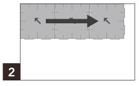
**Starting from a corner,** place the *Ekösteps*® insulating tiles with the *Ekösteps*® logo facing up. To assemble your first row of *Ekösteps*® insulating tiles, simply lock the tongues into the grooves of the previous tile.
