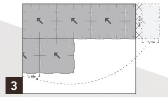
To install your last tile, you may need to cut it with a utility knife. The tiles are embossed with 1 in squares to simplify this task. **Make sure the arrows of all tiles are pointing in the same direction.** If the off-cut of your last *Ekösteps*® insulating tile is at least 12 in, you can reduce losses by starting the next row with a half-tile (12 in) and install them in a staggered pattern (*like a brick wall*). Otherwise, the layout of the tiles will be the same for each row.
